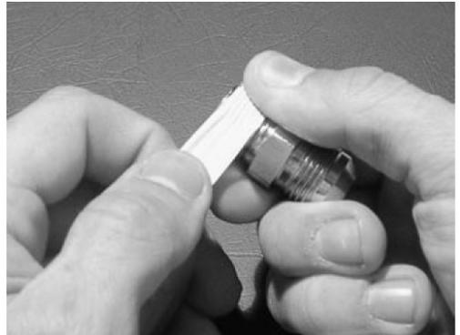
3. Wrap the Teflon tape (3) times around the fitting, hold down on the threads with your thumb, and pull on the tape roll to 'cut' the tape. Don't allow the tape to fray. You now have a properly wrapped fitting ready for use. Install the fitting hand tight, and then give it up to two turns with a wrench. If it wants to stop before two turns, DO NOT force the fitting. You can damage the threads or destroy the seal. Do not back off on a tightened fitting or it might leak.
