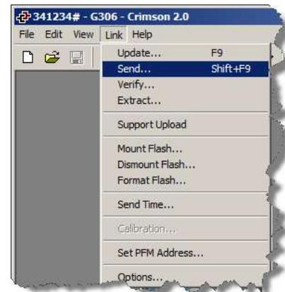
3.9 The transfer to the display will begin. During this time the display will stop running the software. The PC software will show a new window as the download process proceeds.
