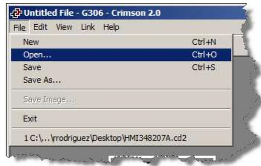
3.7 A new window appears that allows browsing. Find the \*.CD2 Display software file. In this example it is on the desktop. Double click the file.
