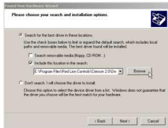
3.3.7 Click on the Browse button to navigate to the driver location on your computer. The location should be C:\Program Files\Red Lion Controls\Crimson 2.0\Device\ if Crimson® 2.0 was installed under the default folder. The OK button can be clicked once a system file is detected in the folder. Click OK.
