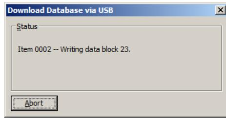
3.10 When the download is complete, the Display will automatically load the new software. Close the Crimson® 2.0 software and disconnect the USB cable.
