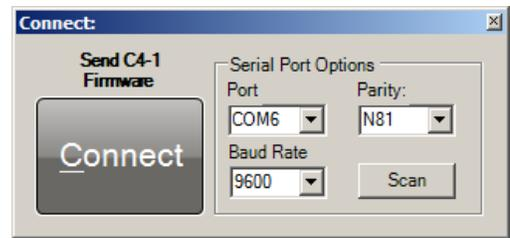
\*If the SCAN button fails to detect the port number, pick the COM port assignment determined by the USB to Serial Bridge manually. **Refer to USB Driver Installation section 1.5 for instructions on determining the correct COM assignment for the PC.**
