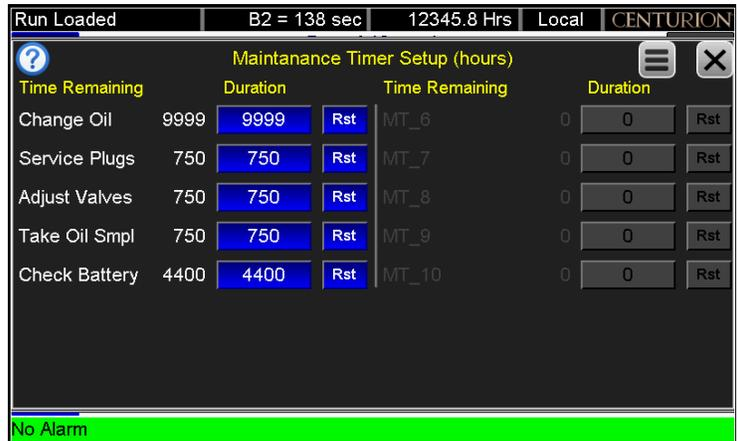
If an interval time has elapsed, a message event is typically used to indicate maintenance is due. Reset the timer after maintenance is performed by pressing the RST icon on this page.
