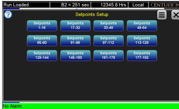
Setpoints are thresholds which can be configured as  $\geq$  or  $\leq$  and analog, temperature, speed or voltage input used for alarms, shutdowns and permissive signals for operating states.
