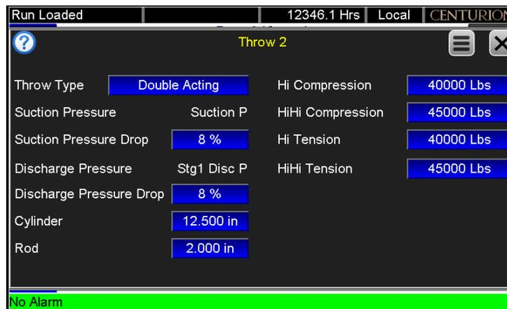
Action may be changed from single to double throw. Set the pressure drop values to approximate internal gas pressures.
