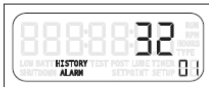
Alarm Code - Shows the Channel Tripped
