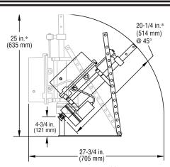
\*These dimensions are given with the CO3 disengaged. When CO3 is engaged, add 6 in. (152 mm).
