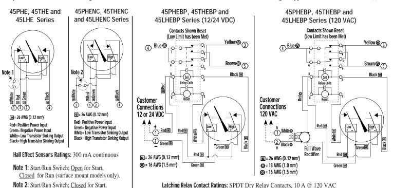
Latching Relay Contact Ratings: SPDT Dry Relay Contacts, 10 A @ 120 VAC
