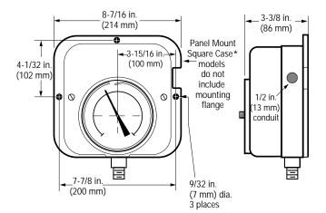
\* 45PHEE, 45LHEE, 45PHENCE, 45LHENCE, 45PHEBPE and 45LHEBPE models feature square case, but altered to fit standard round panel mounting-not pictured.
