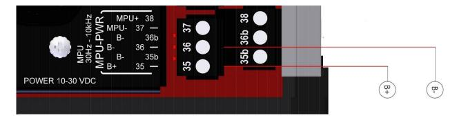
NOTE: Run power directly from battery posts to controller power terminals when battery is the power supply.
