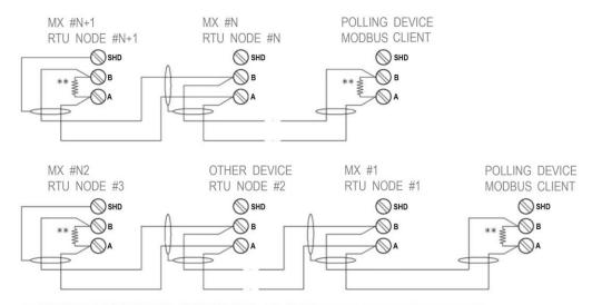
\*\* USE EIA RS485 SHIELDED, TWISTED PAIR, 120 OHMS CHARACTERISTIC IMPEDANCE.
