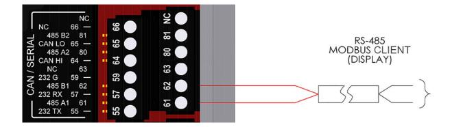
**NOTE**: A is the non-inverting pin and should have a single pull-up physically placed anywhere on the network. B is the inverting pin and should have a single pull-down physically placed anywhere on the network.
