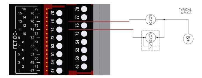
**NOTE**: If an inductive load does not have an internal flyback diode, it is recommend you install a 1A 600V PIV diode in parallel with the load. (1N4005 – EC P/N 36-16-1002)
