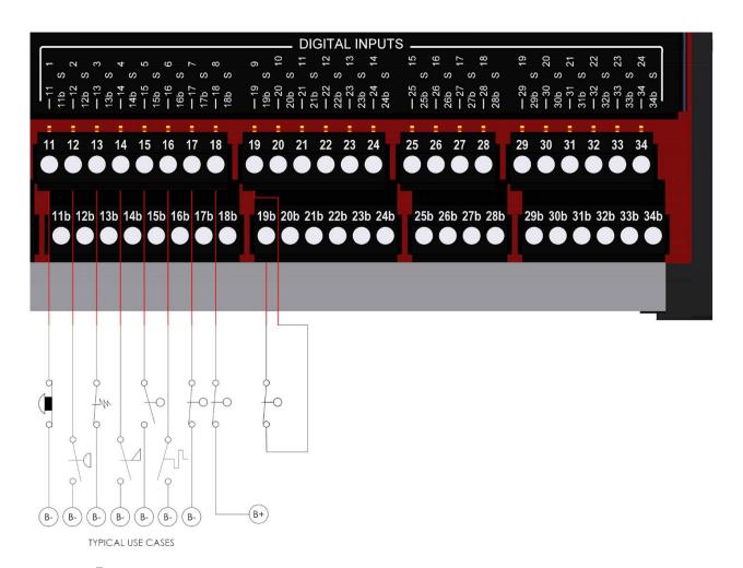
**NOTE**: These circuits are not required to be in conduit if all the requirements for ic protection are met and Authority Having Jurisdiction (AHJ) allows.
