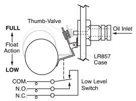
As the equipment uses oil, the float falls, providing immediate level compensation. At FULL position, the float holds the valve closed. If the clean oil supply is depleted and oil level continues to fall, the low level switch will operate an alarm or equipment shutdown.
