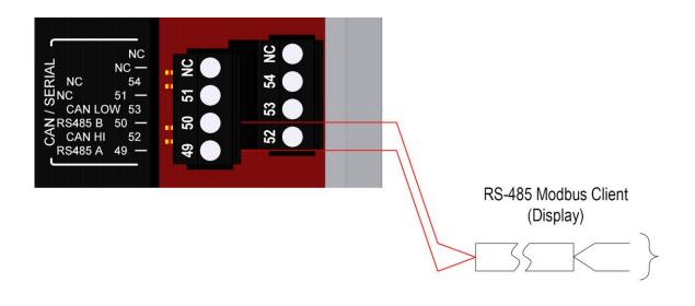
**NOTE**: A is the non-inverting pin and should have a single pull-up physically placed anywhere on the network. B is the inverting pin and should have a single pull-down physically placed anywhere on the network.
