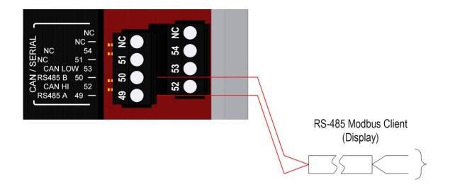
**NOTE**: A is the non-inverting pin and should have a single pull-up physically placed anywhere on the network. B is the inverting pin and should have a single pull-down physically placed anywhere on the network.
