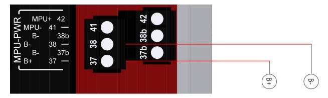
NOTE: Run power directly from battery posts to controller power terminals when battery is the power supply.
