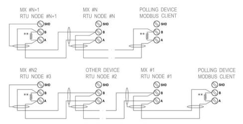
\*\* USE EIA RS485 SHIELDED, TWISTED PAIR, 120 OHMS CHARACTERISTIC IMPEDANCE. INSTALL 120 OHMS TERMINATING RESISTOR ON FIRST AND LAST NODE ON RS-485 NETWORK. ALL RS-485 DEVICES MUST SHARE DC COMMON GROUND.
