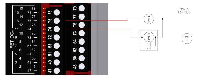
**NOTE**: If an inductive load does not have an internal flyback diode, it is recommend you install a 1A 600V PIV diode in parallel with the load. (1N4005 – EC P/N 36-16-1002)
