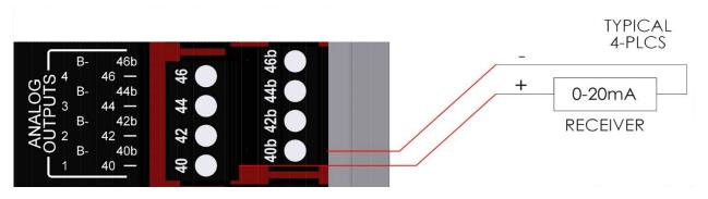
NOTE: The MX5-R2 provides all operating power (~B+) to the transmitter and receiver and any other loop components.
