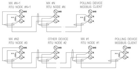
\*\* USE EIA RS485 SHIELDED, TWISTED PAIR, 120 OHMS CHARACTERISTIC IMPEDANCE. INSTALL 120 OHMS TERMINATING RESISTOR ON FIRST AND LAST NODE ON RS-485 NETWORK. ALL RS-485 DEVICES MUST SHARE DC COMMON GROUND.
