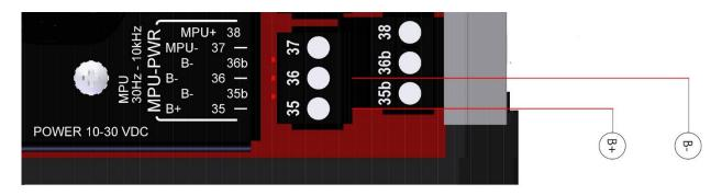
NOTE: Run power directly from battery posts to controller power terminals when battery is the power supply.
