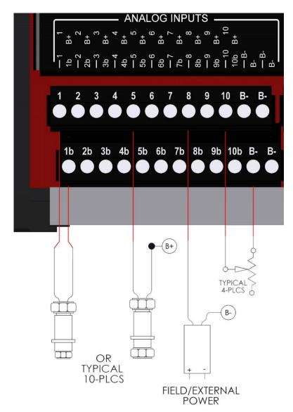
**NOTE**: These circuits are not required to be in conduit if all the requirements for ic protection are met and Authority Having Jurisdiction (AHJ) allows.
