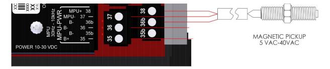
**NOTE**: The MPU input requires a minimum signal of 2 Vrms when connected.
