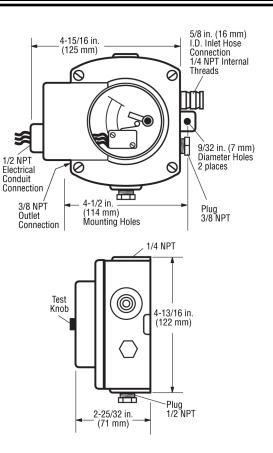
FW Murphy offers two mounting brackets for the LR857. The 15000238 Pipe Bracket Kit fits a 7/8 in. (22 mm) diameter pipe (see typical installation). The 15010224 universal Flange Kit allows various mounting methods.
