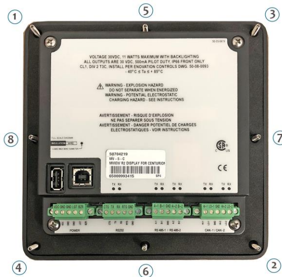
Backside of MV-5-C showing gasket, studs and tightening sequence
