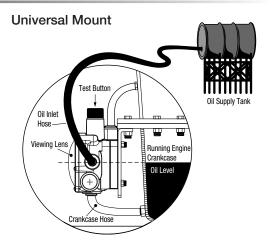
In addition to the direct mounting option, FW Murphy offers two mounting brackets for the LM500. The pipe bracket fits a 7/8 in. (22 mm) diameter pipe. The universal bracket allows various mounting methods. For exact dimensions visit, http://www.fwmurphy.com.
