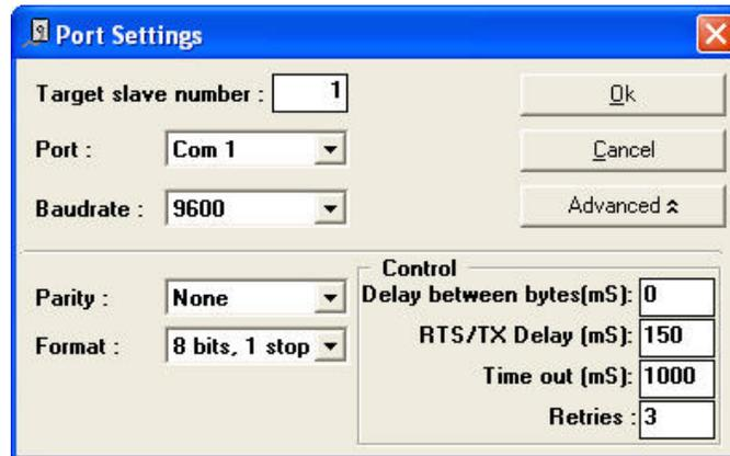
**The TTD will not accept Modbus writes for some registers while in the Run Mode. To perform a complete Download, it is necessary to be in Shutdown Mode on the TTD.**
