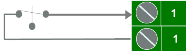
Normally closed sensor wiring to TTD (typical)
