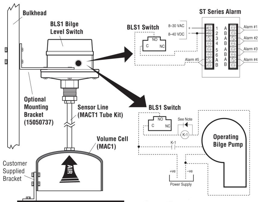
NOTE: Contact rating should be appropriate for horse power of the pump.
