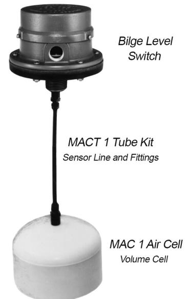
As bilge level rises, a column of air is captured in the MAC1 Air Volume Cell. The rising bilge level compresses the column of air creating pressure against the large diaphragm in the BLS1 Bilge Level Switch and the switch trips. Switch set point is adjustable.
